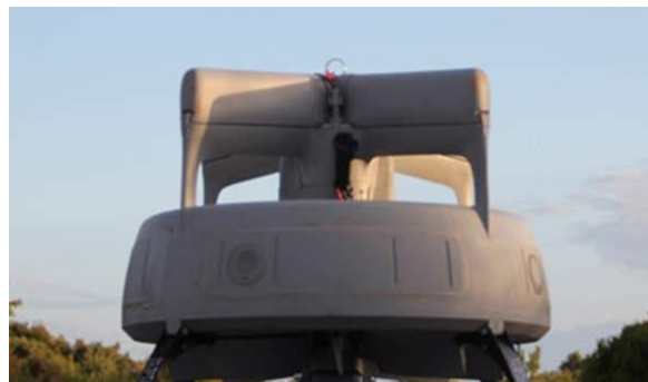
Figura 5: Spyball-B Micro Unmanned Aerial System (MUAS) - www.army-technology.com
